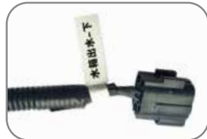
Radiator outlet sensor
